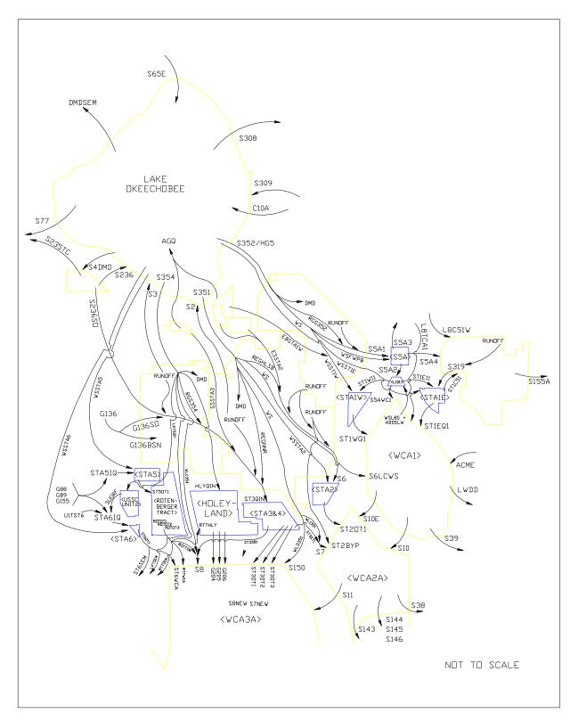
**Figure 3.3.7** Flow Distribution Within and Around the Everglades Agricultural Area with the Proposed Stormwater Treatment Areas In Place as Implemented in the South Florida Water Management Model
