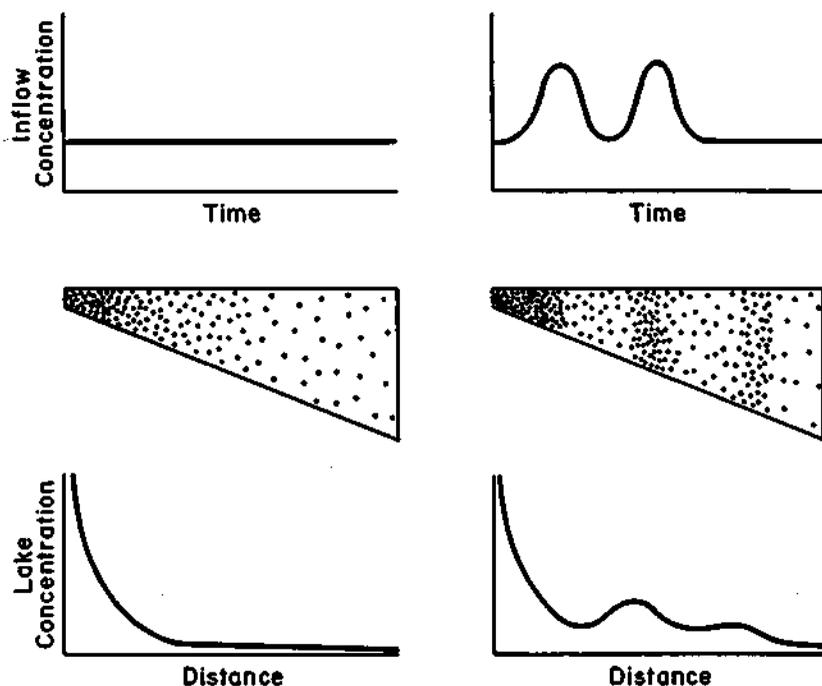
Figure 5.3 Material distributions along a reservoir receiving inflows with constant concentration (left) and a similar reservoir receiving inflows with variable concentration (right).
