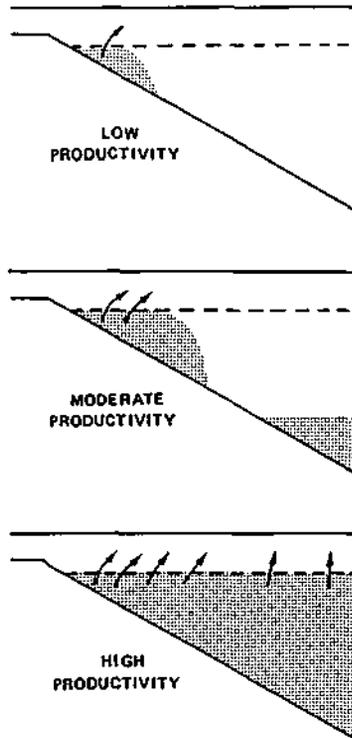
**Figure 5.9** Longitudinal occurrences of hypolimnetic anoxia and nutrient increases (shading), and upward exchanges of nutrients (arrows) in reservoirs of differing productivity and loading.
