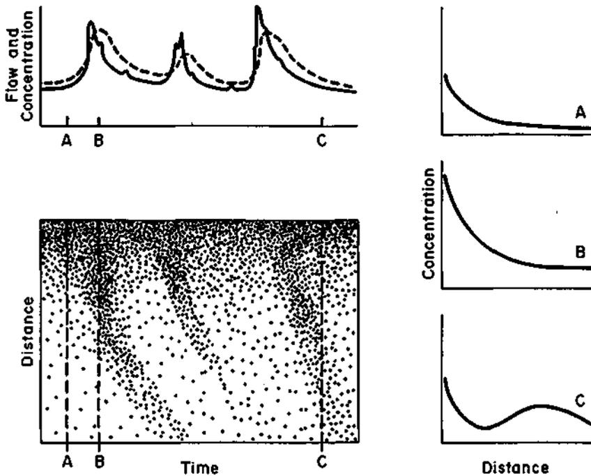
Figure 5.4 The combined effects of changes in tributary concentration and flow (upper left) on the spatial and temporal distribution of materials (shading) in the receiving reservoir (lower left). Longitudinal gradients in material concentration observed at three points in time (A, B, and C) are also depicted (right).
