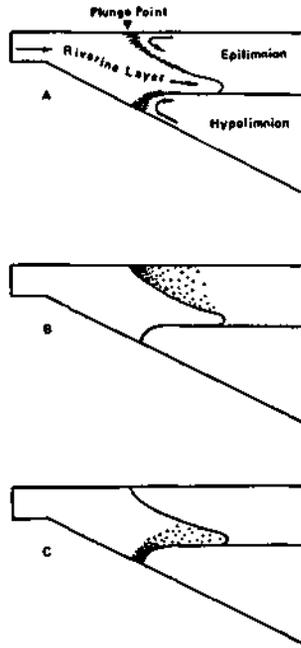
**Figure 5.6** Turbulent interfaces (zigzag line) between epilimnion, hypolimnion, and an interflowing riverine layer (a). Exchanges of material from riverine layer to epilimnion (b) and from hypolimnion to riverine layer (c) are also indicated (shading).
