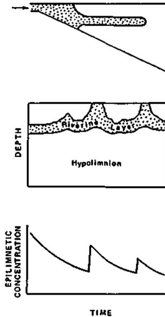
**Figure 5.7** The effects of internal mixing of nutrient-rich riverine water (shading) and epilimnetic water on epilimnetic nutrient concentrations (based on Carmack and Gray 1982).
