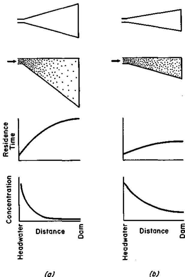
Figure 5.2 Distribution of inflow material (shading) and changes in water residence time and material concentration with distance from headwater to dam in two reservoirs receiving similar input but differing morphologic characteristics, one broad and deep (a) and the other narrow and shallow (b).
