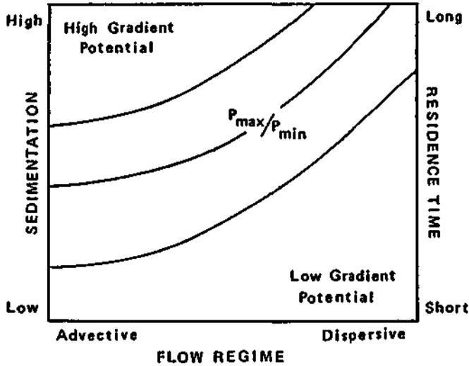
Figure 5.5 The dependence of phosphorus gradient potential on sedimentation rate, residence time, and flow regime. Lines of equal  $P_{max}/P_{min}$  (the ratio of maximum to minimum observed phosphorus concentration) are plotted. (Based on Walker 1982a.)
